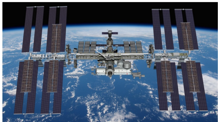
Figure 1: iROSA deployed over top of the ISS original solar arrays.
